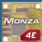
Monza 4E tag chips offer up to 496 bits of EPC memory, 128 bits of User memory, and a serialized TID to provide fast access to a larger memory, as well as meet the
