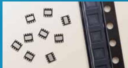
Monza 4 tag chips encapsulated in 8-pin  $\mu$ DFN packages accommodate surface-mount assembly and enable ruggedized tag designs.
