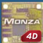
Monza 4D tag chips provide 128 bits of EPC memory, 32 bits of User memory, and a serialized TID. For applications where large memory is not required,
