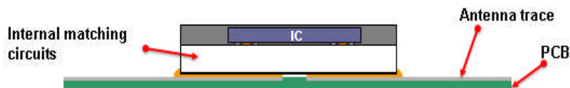
Figure 2: Cross-section of Murata MAGICSTRAP®
